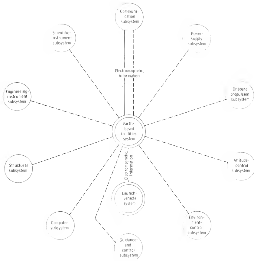
FIGURE 7-1.—Interface diagram showing the more important relationships between the Earth-based facilities and the rest of the satellite system. The dotted lines represent prelaunch testing and checkout relationships; the solid lines show postlaunch interfaces.
